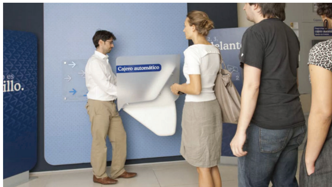
IDEO has designed an ATM for Spanish bank BBVA, which uses touchscreen technology and angles the machine at 90 degrees, a departure from conventional ATMs.
